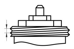
Note on determing screw lead: Measure the distance between thread transitions. They have 1mm or 1.5mm.
